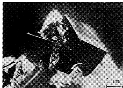
Fig. 5. Cubic crystal grown on the tip of tungsten wire.
